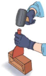
A club hammer and brick bolster are used to cut bricks
